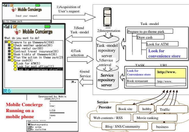
Fig.1 Architecture of task based service navigation system
