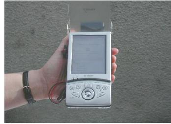
Fig. 6. PDA with wireless card and location receiver.
