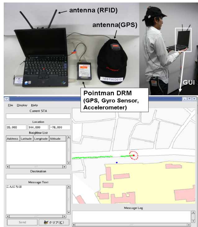
Fig.1 Brief sketch of the implemented system. We can utilize GPS where it is available. Otherwise, we use only the information from RFID, gyro sensor, accelerometer and location information (with estimated error) of neighbor person who is in the range of wireless receiver/transmitter.
